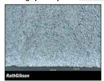
Transverse section of RathGibson laser welded 0.083" (2.11 mm) average wall tubing. The tube's ID surface is visible at the bottom. Note the weld recrystallization and the ID weld.
