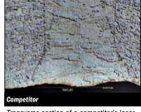
Transverse section of a competitor's laser welded 0.065" (1.65 mm) average wall tubing. The tube's ID surface is visible at the bottom. Note no discernable recrystallization or cold work and the ID is unforged.
