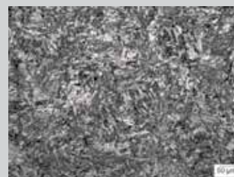
Figure 1. Typical P92 Microstructure
