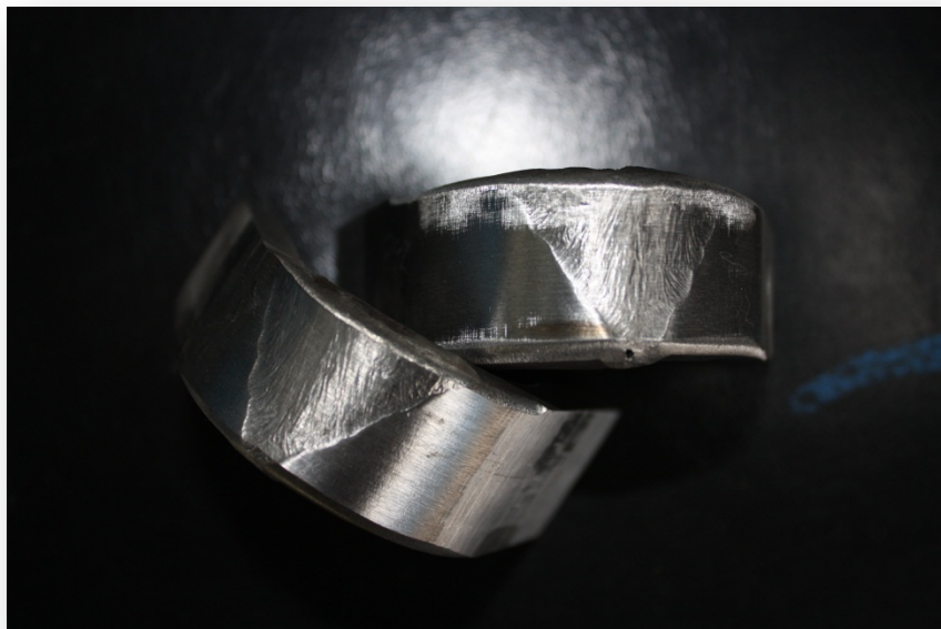
Figure 21. Photograph Illustrating Acceptable Direct Aged 2T Side Bends Utilizing SMAW to Join Alloy 740H to P92 Steel with INCONEL 182 Welding Electrodes.
