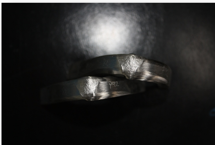
Figure 21. Photograph Illustrating Acceptable Direct Aged 2T Side Bends Utilizing SMAW to Join Alloy 740H to P92 Steel with INCONEL 182 Welding Electrodes.
