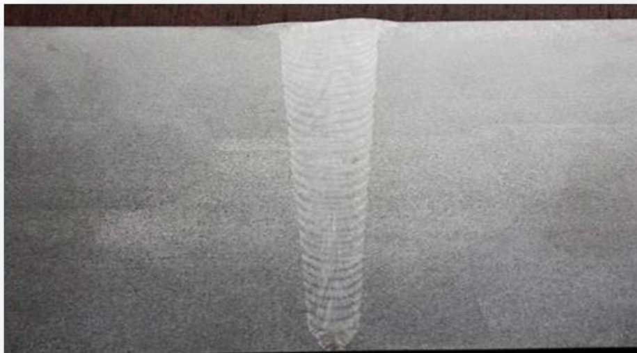
Figure 16. Etched cross section of a HWGTA weldment in 3" wall INCONEL alloy 740H steam header tube weldment showing bead sequence.
