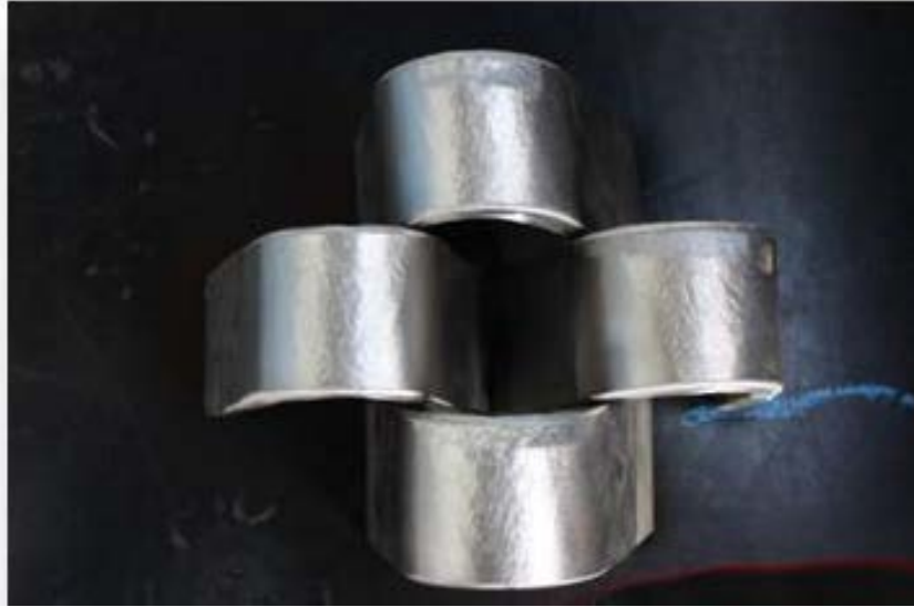
Figure 19. 2 inch (50.8mm) full section p-GMAW 2T side bend tests.
